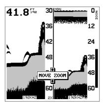
shown on the left side of the screen. Pressing the up or down arrow keys moves the zoom bar up or down. As you adjust the zoom bar, the range changes on the left side of the screen at the same time.
